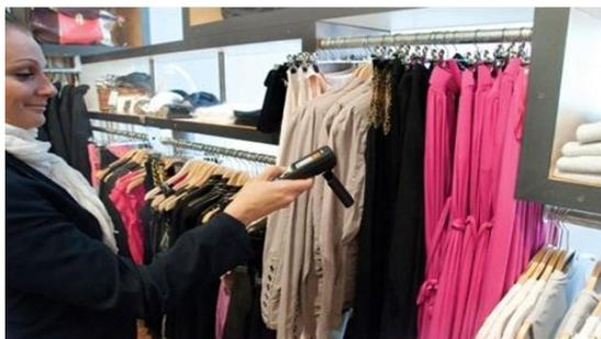
**Fig.:** RFID detector detecting the RFID tags
